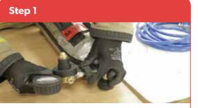
Pick up part 2 and screw part 2 into the threaded valve of part 1. The connection should be hand tight only.
