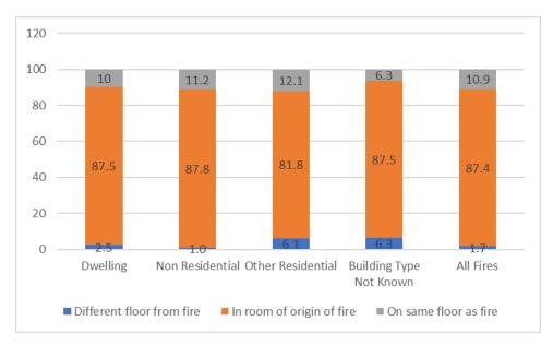
Figure 5: Location of Sprinkler System where System Operated by Building Type, %
