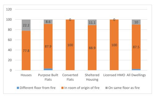
Figure B3: Location of Sprinkler System where System Operated by Dwelling Type, %
