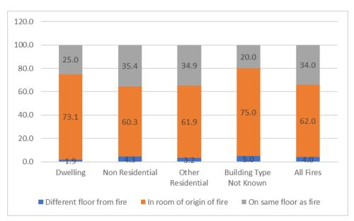
Figure 9: Location of Sprinkler System where System did not Operate by Building Type, %
