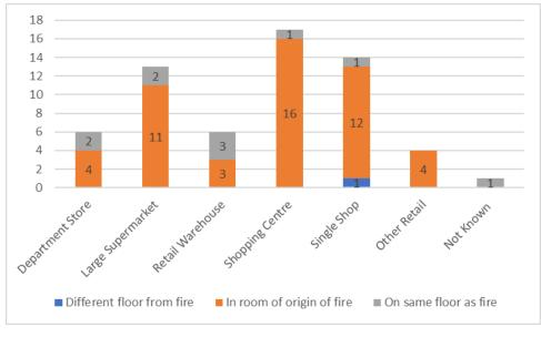
Figure C11: Location of Sprinkler System where System Operated, Retail Sub-Sectors
