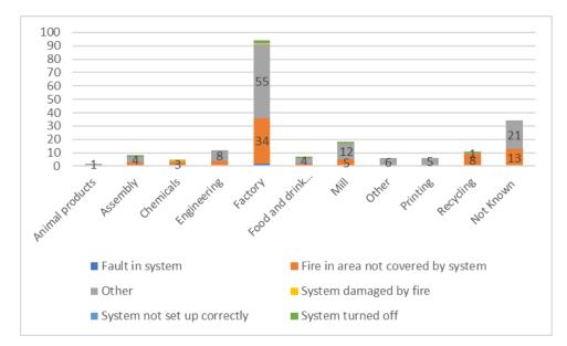
Figure C8: Reaons for Sprinkler System not Operating, Industrial Fires by Sub-Sector
