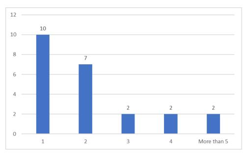
Figure C20: Number of Fires by Number of Heads Activated, Warehousing and Bulk Storage Sub-Sectors
