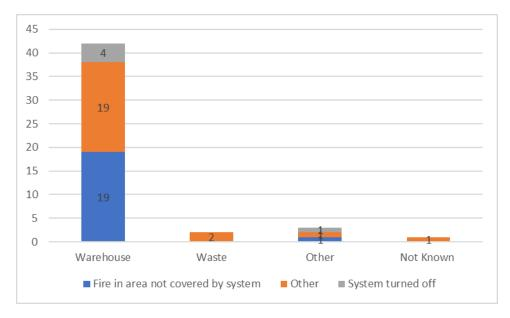
Figure C24: Reasons why Sprinkler System did not Operate, Warehousing and Bulk Storage Sub-Sectors
