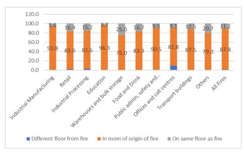
Figure B11: Location of Sprinkler System where System Operated by Non-Residential Sector, %
